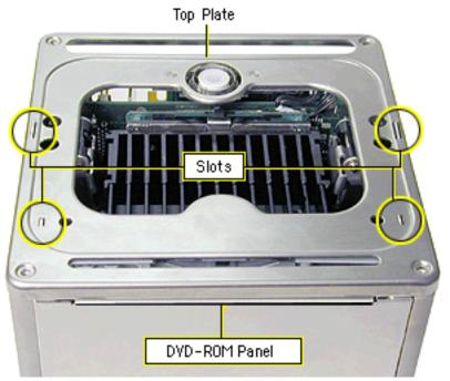
4. Starting with the four corner screws, secure the top plate to the core with all eight screws.
